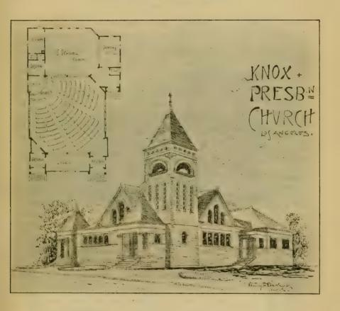
This is a substantial frame building, erected in Los Angeles, Cal., at an expense of about \$3,500. The main audience room is 45x45, seating about 350, and the lecture room 30x30. The entire capacity of the building, when all the rooms are thrown together, would be about 500. The architect is Mr. H. F. Starbuck.
